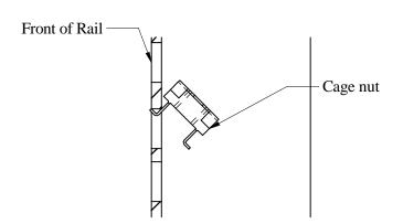
**STEP 1:** Locate cage nut as shown on back side of rail.
