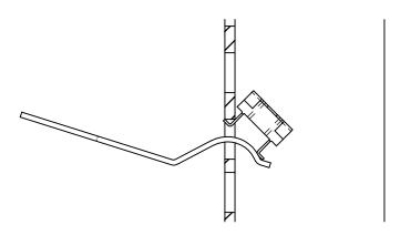
STEP 2: Insert through hole and hook onto bottom lip of cage nut.
