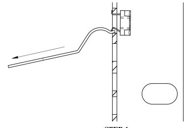
STEP 4: As you rotate down pull the tool back through the hole.
