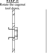
Cage nut fully positioned
